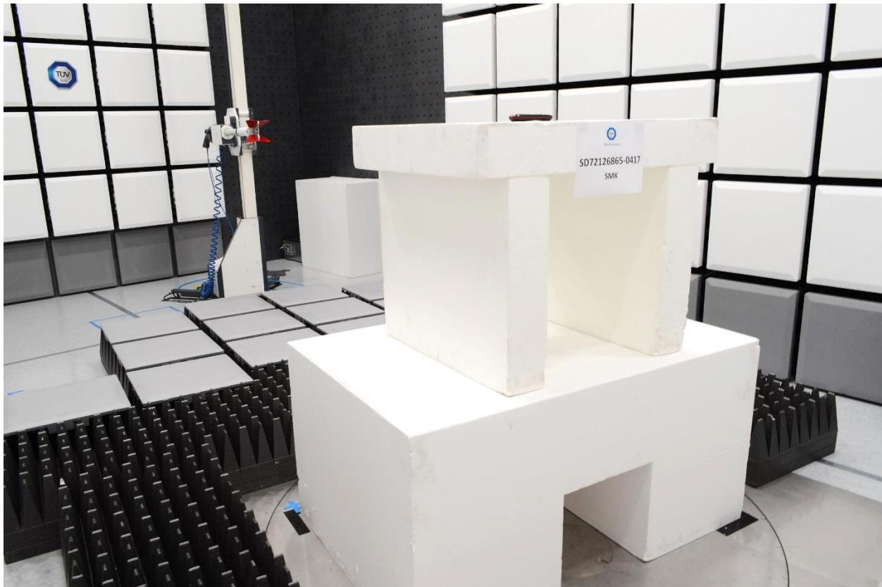
**Radiated Emissions Test Setup (above 1GHz Back)**
