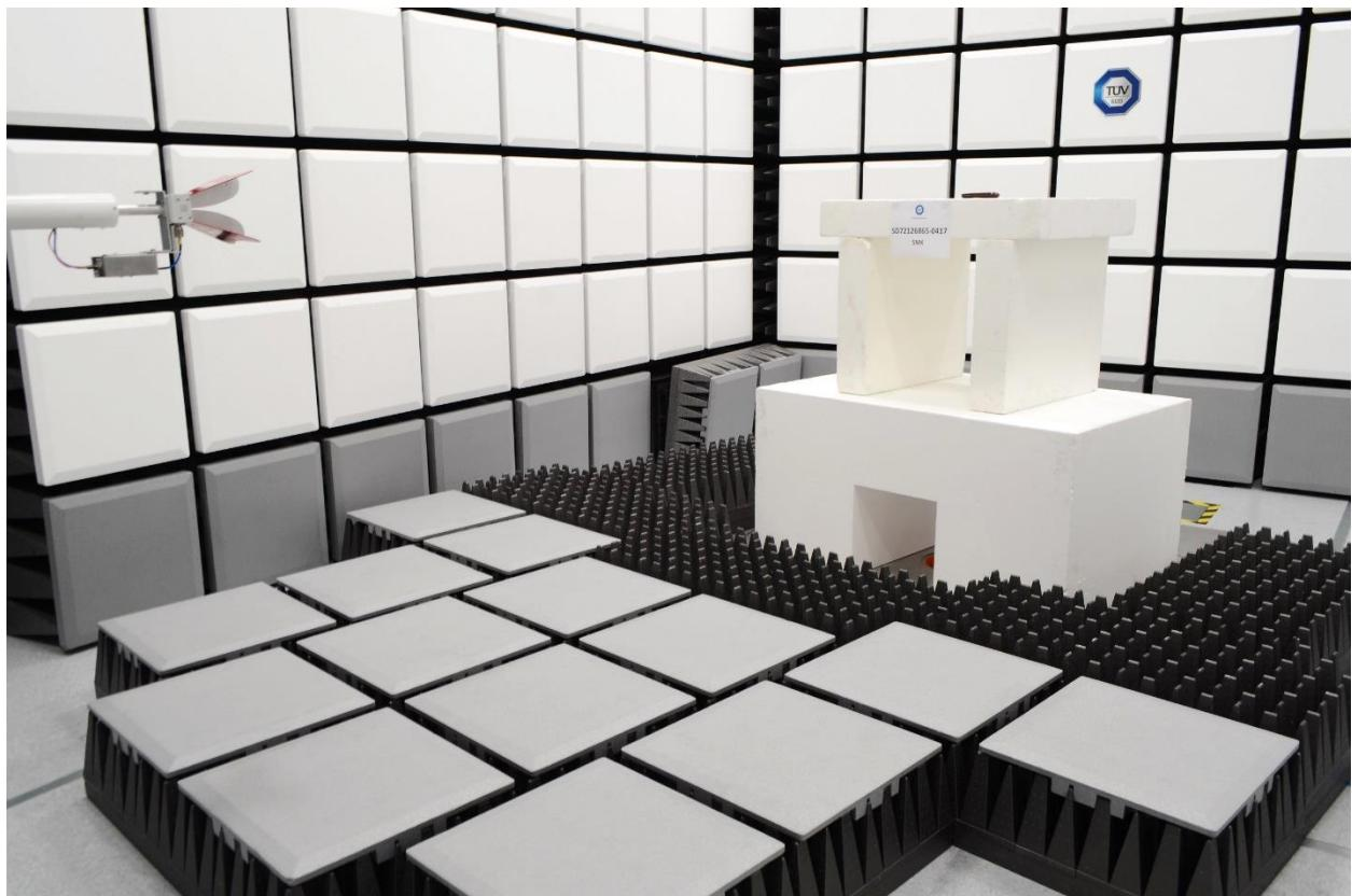
**Radiated Emissions Test Setup (above 1GHz Front)**
