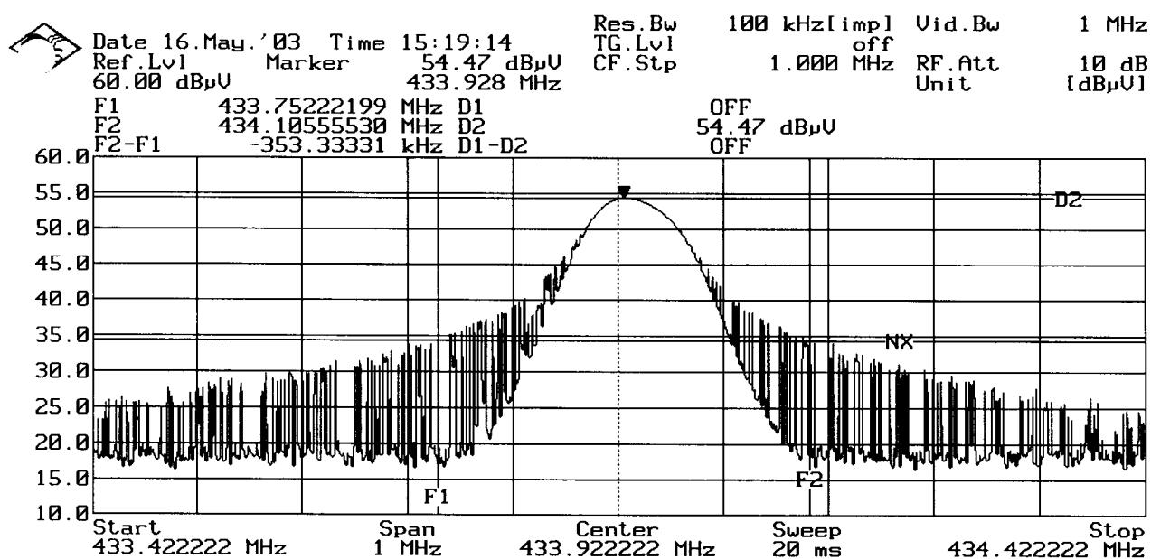
The measured 20 dB bandwidth is: .....353.3 kHz
