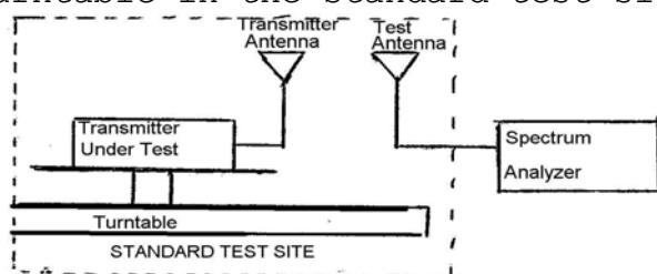
b) Raise and lower the test antenna from 1m to 6 m with the transmitter facing the antenna and record the highest received signal in dB as LVL.
