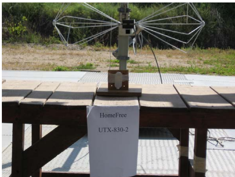
Figure 3. Radiated Emission Test 30 MHz – 1000 MHz
