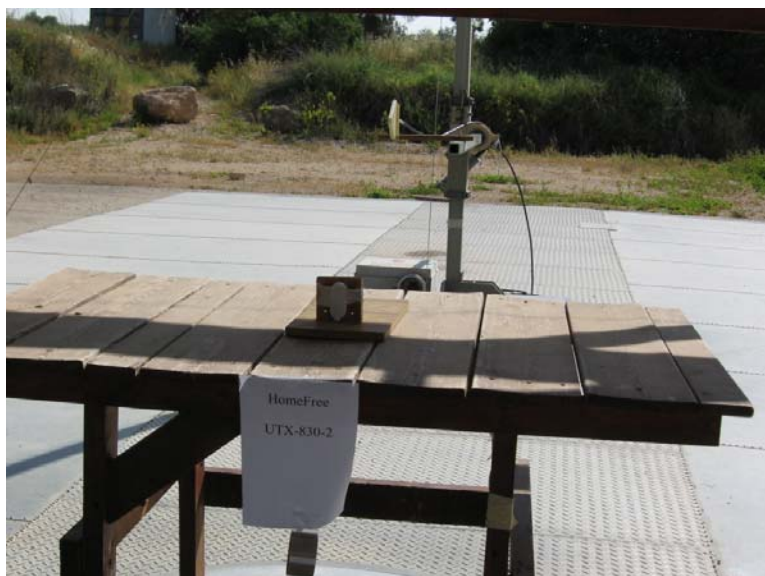
Figure 4. Radiated Emission Test Above 1000 MHz
