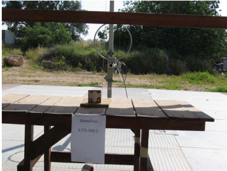
Figure 2. Radiated Emission Test 9 kHz – 30 MHz
