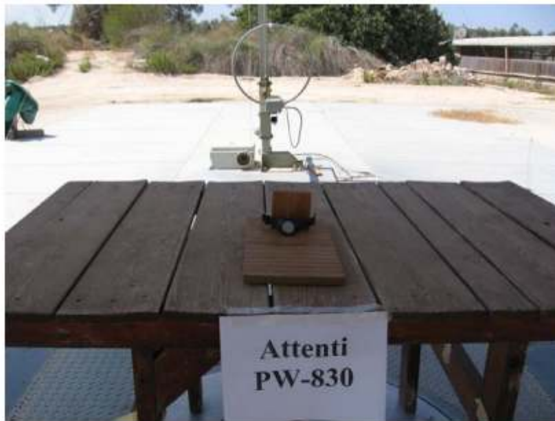
Figure 2. Radiated Emission Test 9 kHz – 30 MHz
