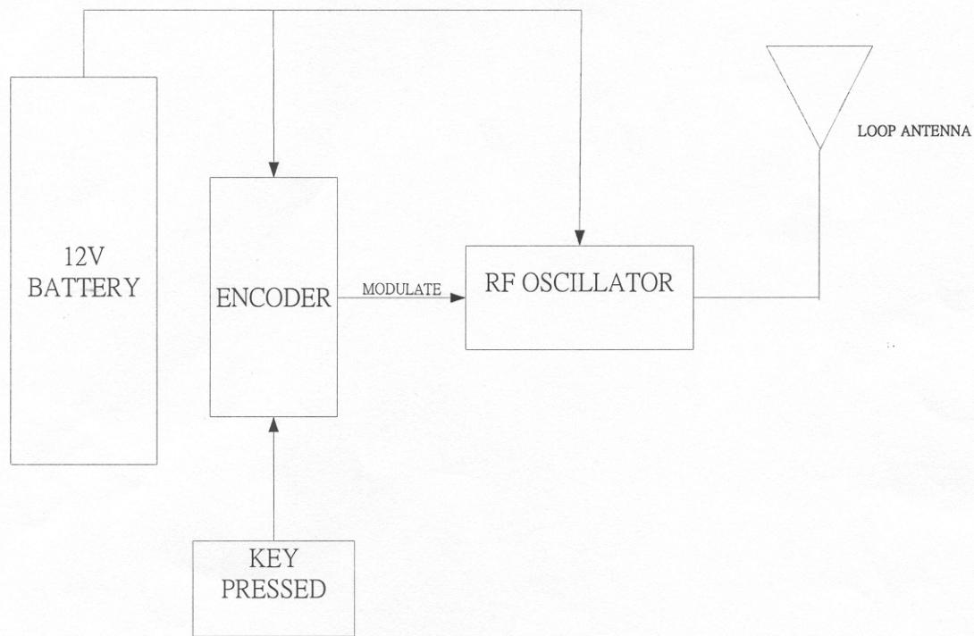
When a key pressed encoder will send a code to activate rf oscillator then transmite a rf signal through antenna.
