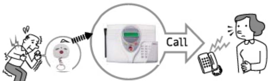
The user presses and holds the red **SOS** button on the Keychain Remote or main controller.
