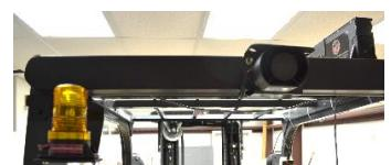
Install the Generator on top of the overhead guard and at least 4" (10.2cm) from the frame if placed on the counterbalance. **It should be as far from the strobe light as possible.** Adjust magnets to fit as needed.
