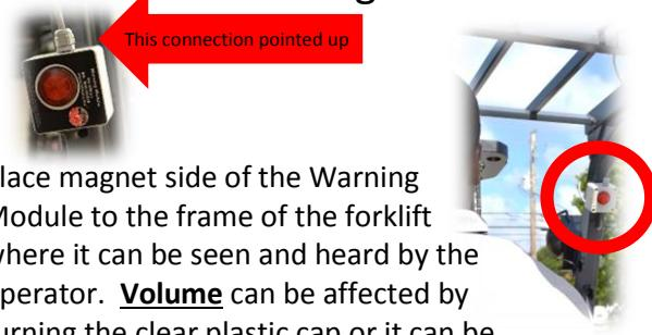
Place magnet side of the Warning Module to the frame of the forklift where it can be seen and heard by the operator. **Volume** can be affected by turning the clear plastic cap or it can be removed.
