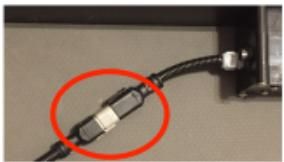
Connect Warning Module (Plug) to Generator (Receptacle).
