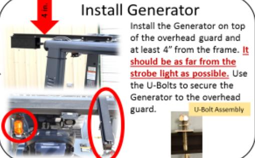
Install the Generator on top of the overhead guard and at least 4" from the frame. **It should be as far from the strobe light as possible.** Use the U-Bolts to secure the Generator to the overhead guard.
