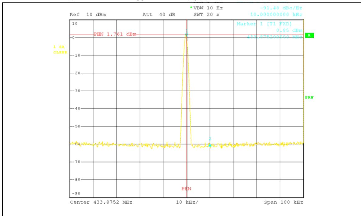
$f_{RF} = 433$  MHz,  $V_{CC} = 3.0$  V,  $R_{MODIN} = 3$  K $\Omega$ , 100 KHz offset
