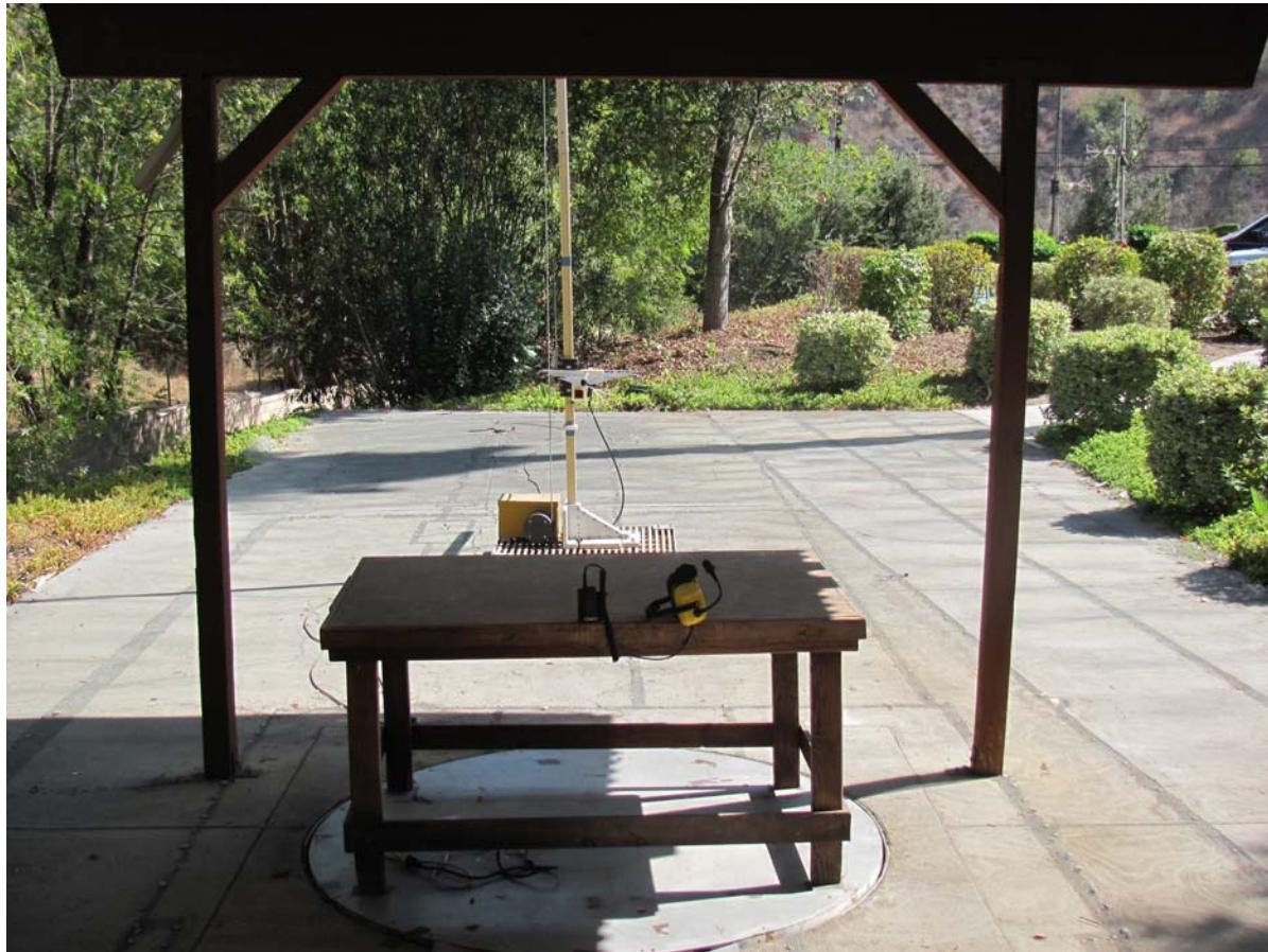
**REAR VIEW****SPECIAL ELECTRONICS & DESIGNS, INC.****FM 916 MHZ TRANSMITTER****MODEL: TT916-TX****FCC SUBPART B AND C – RADIATED EMISSIONS****PHOTOGRAPH SHOWING THE EUT CONFIGURATION
