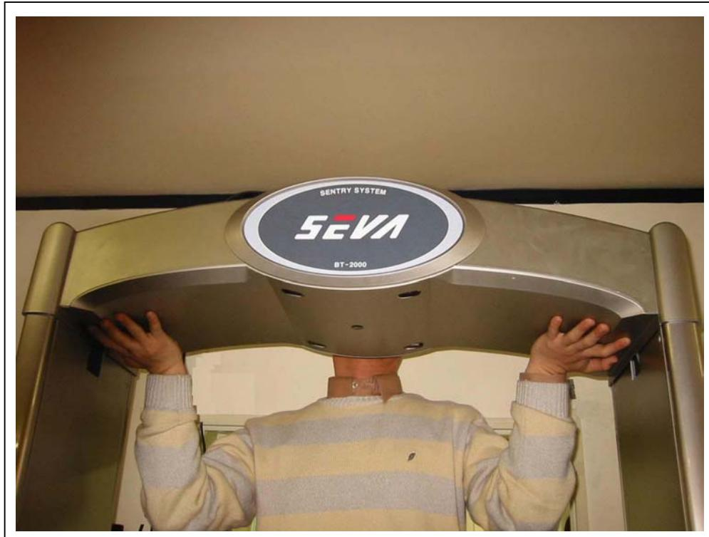
4-8. Place 4x60mm bolts and 5mm washers (4 places-each side) to the bridge to connect bridge and side panels. Make sure stainless steel stiffener is placed.
