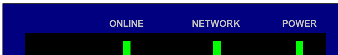
Figure 1: The Point-M access point has 3 LEDs that provide status information.
