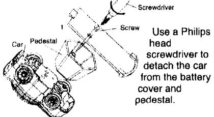
Use a Philips head screwdriver to detach the car from the battery cover and pedestal.
