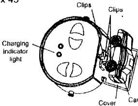
To make the car go, push the forward or reverse button. The car will turn left and right when the left and right button is pushed. The car will only turn left and right when it is moving in forward or reverse direction. The operating light will come on when car is in use. When indicator light becomes faint, it is time to replace batteries. While operating controller, make sure antenna is fully extended.
