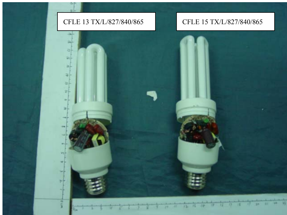
FIGURE 4 Energy Saving Lamp Cover Removed
