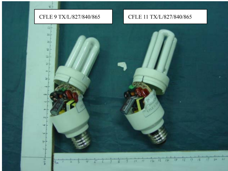
FIGURE 3 Energy Saving Lamp Cover Removed
