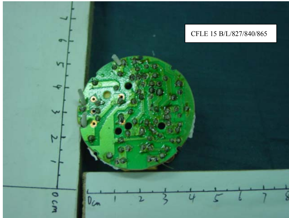
FIGURE 13 Energy Saving Lamp Main Board (Soldered Side)
