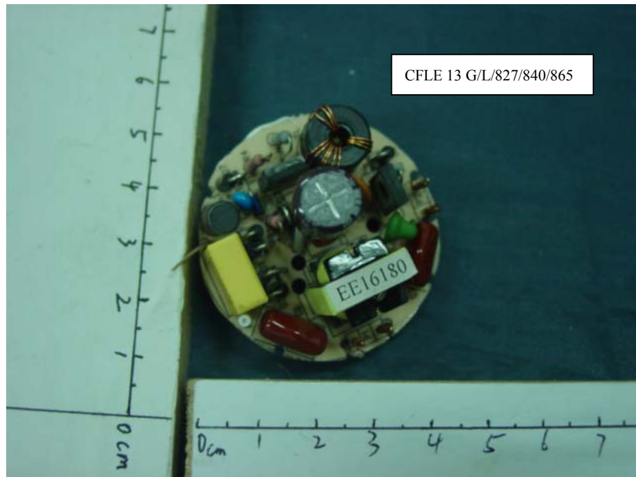
FIGURE 14 Energy Saving Lamp Main Board (Component Side)
