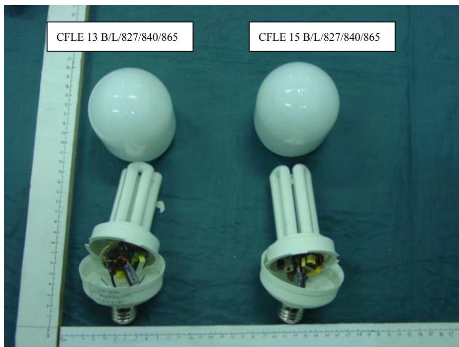
FIGURE 2 Energy Saving Lamp Cover Removed
