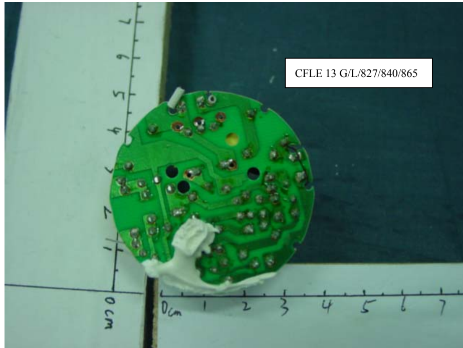
FIGURE 15 Energy Saving Lamp Main Board (Soldered Side)
