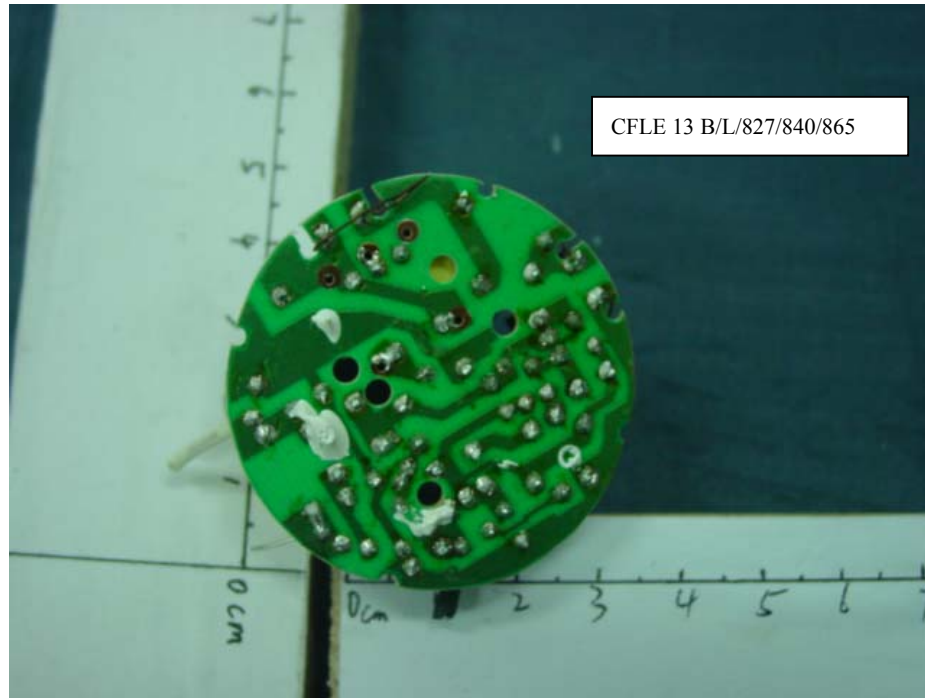
FIGURE 11 Energy Saving Lamp Main Board (Soldered Side)
