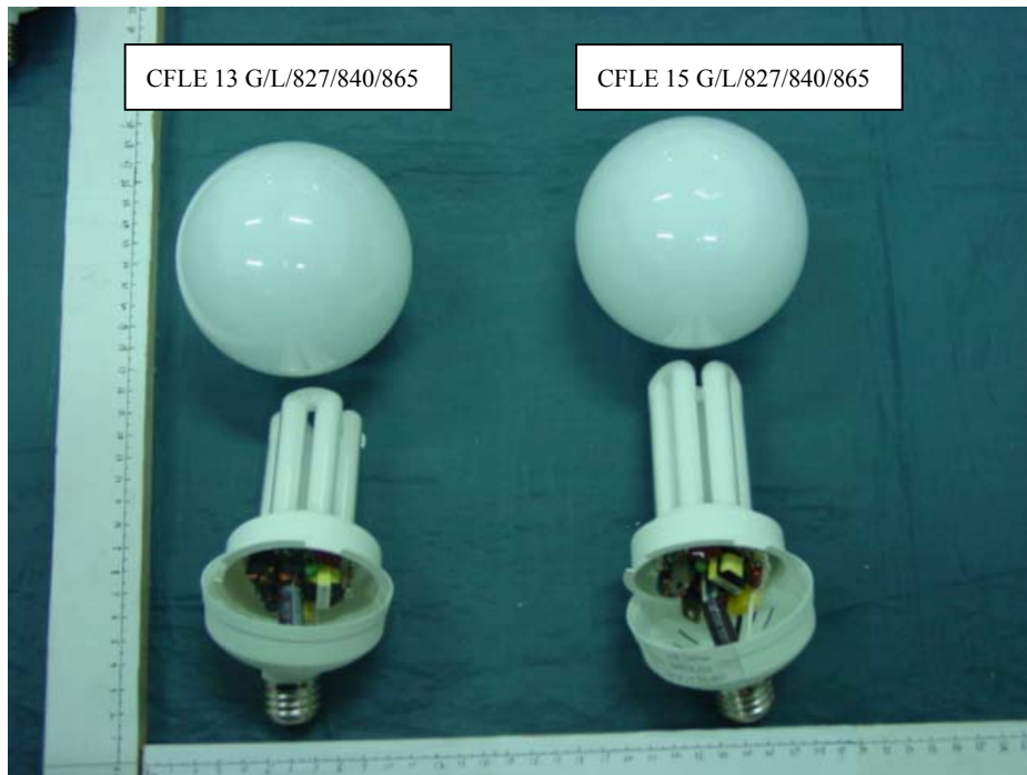
FIGURE 3 Energy Saving Lamp Cover Removed
