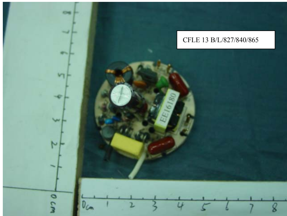
FIGURE 10 Energy Saving Lamp Main Board (Component Side)
