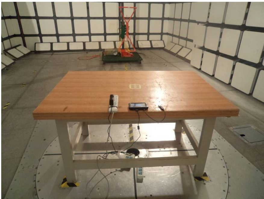
Radiated Emissions-Rear View (30-1000 MHz)
