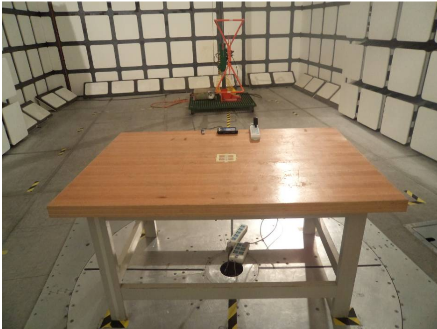
Radiated Emissions-Front View (30-1000 MHz)
