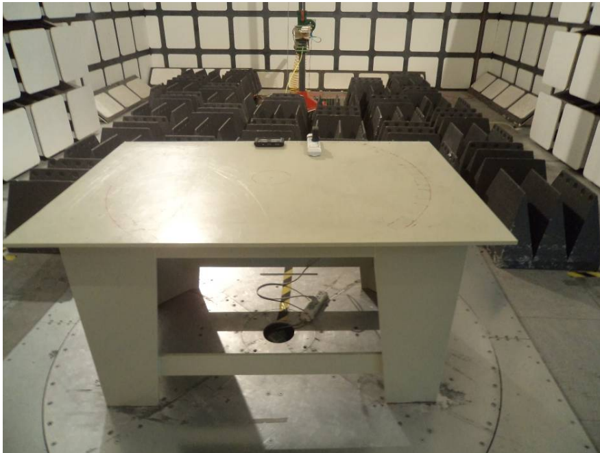
Radiated Emissions –Front View (Above 1GHz)
