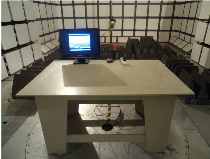
Radiated Emissions-Front View (Charging&Playing&HDMI Output, 1000-6000 MHz)
