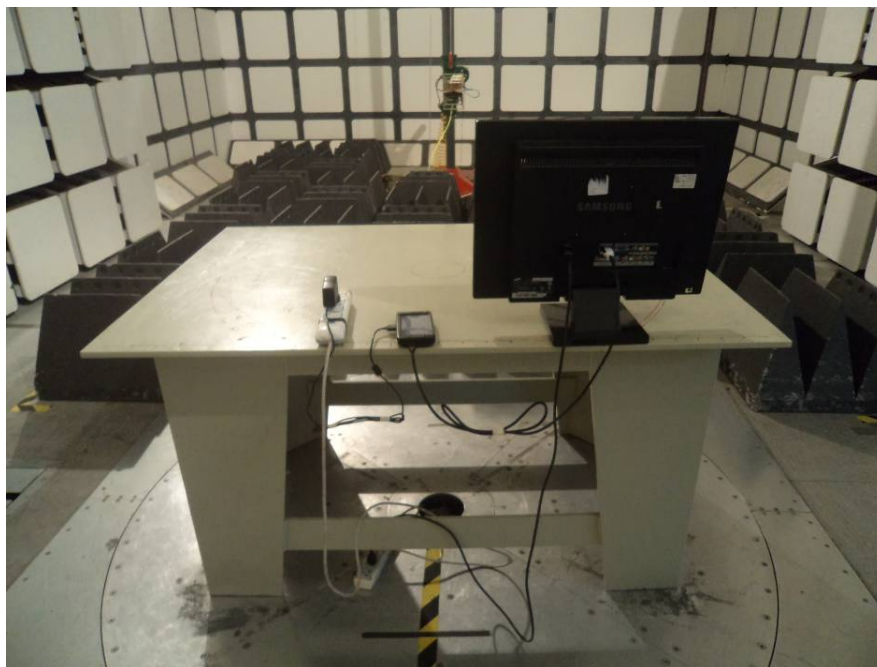
Radiated Emissions-Front View (Charging&Playing&HDMI Output, 1000-6000 MHz)
