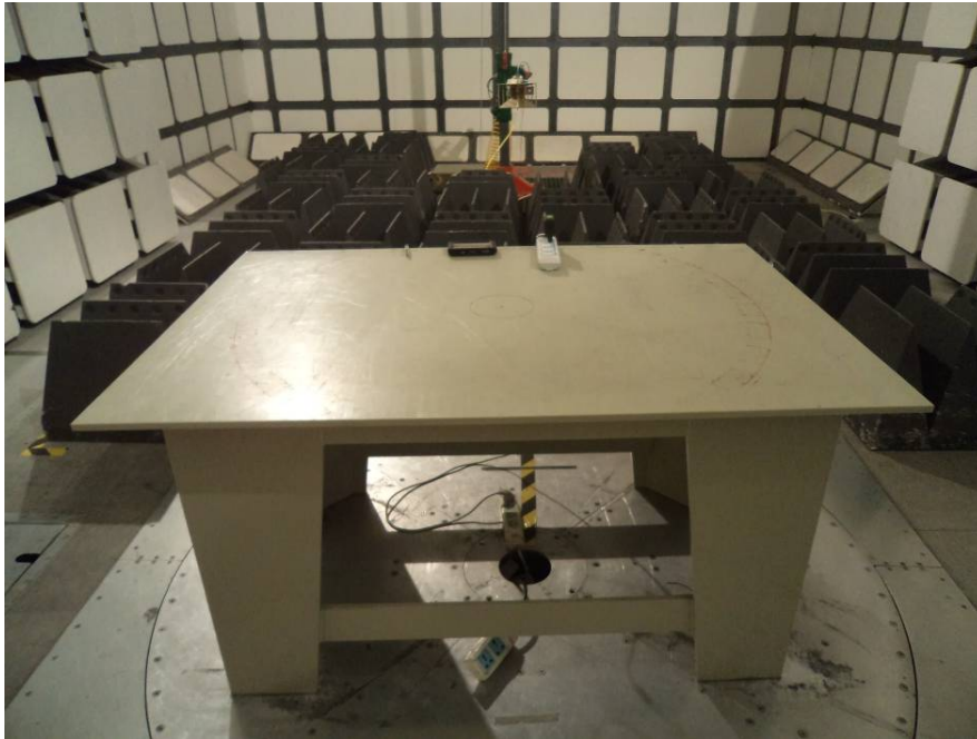
Radiated Emissions- Rear View (Running&Data transmitting with USB disk, 1000-6000 MHz)
