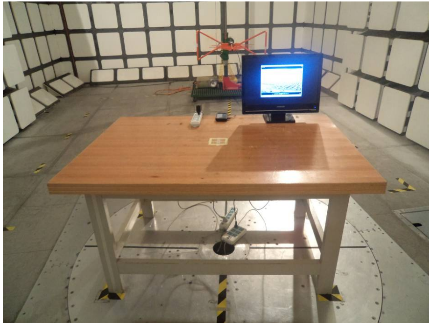
Radiated Emissions-Front View (Charging&Playing&HDMI Output, 30-1000 MHz)
