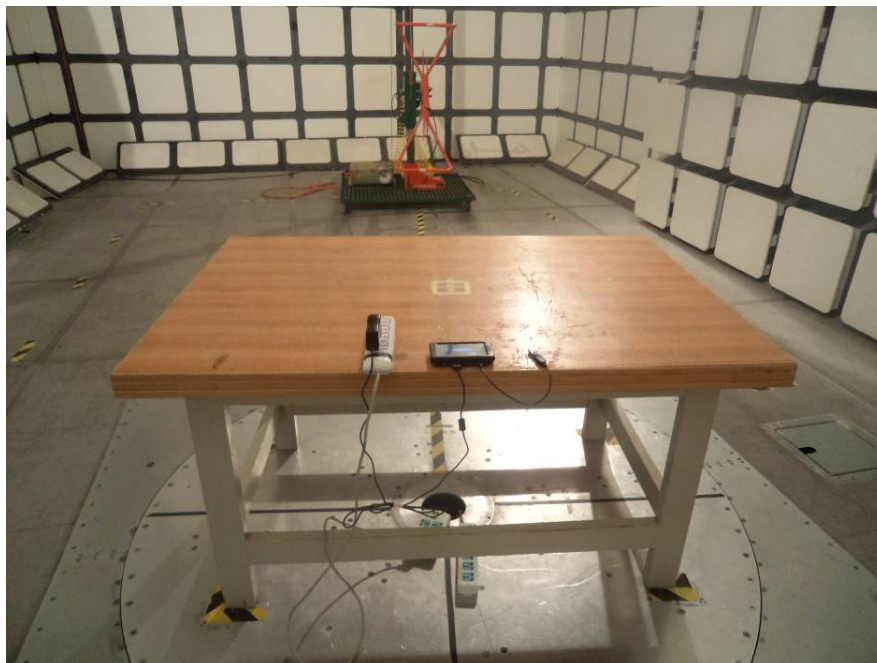
Radiated Emissions – Rear View (Running&Data transmitting with USB disk, 30-1000 MHz)
