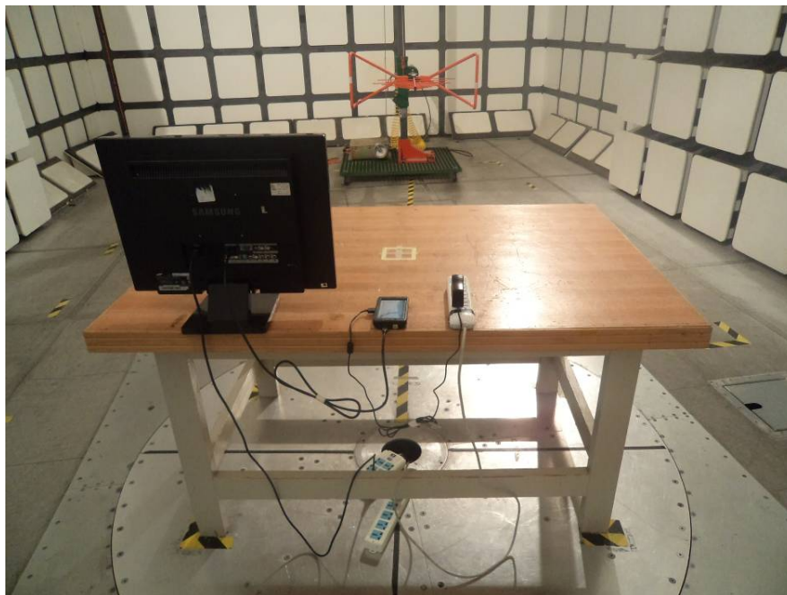
Radiated Emissions – Rear View (Charging&Playing&HDMI Output, 30-1000 MHz)
