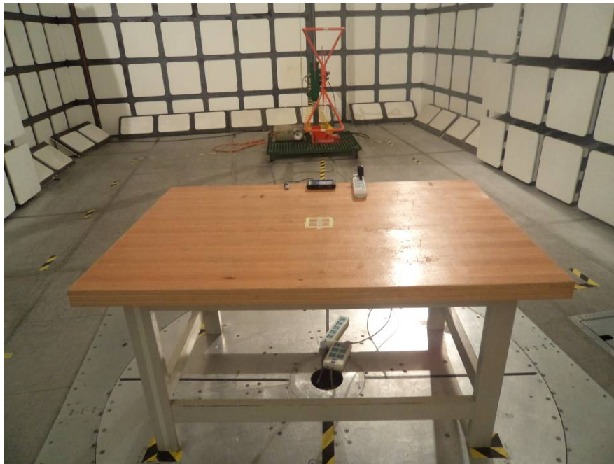
Radiated Emissions-Front View (Running&Data transmitting with USB disk, 30-1000 MHz)
