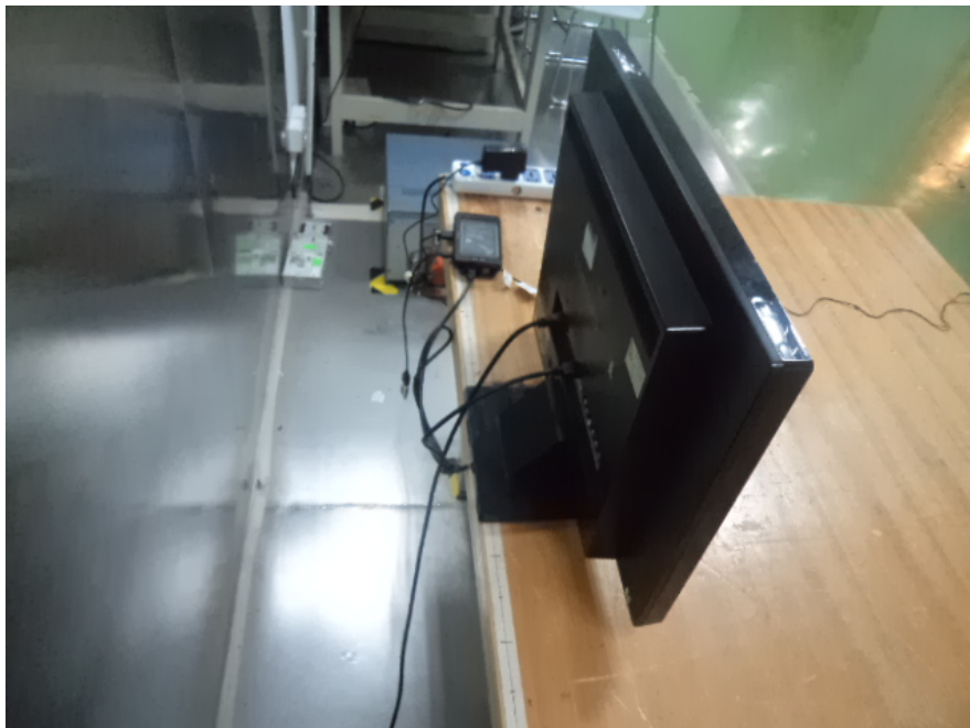
Conducted Emissions - Side View (Charging&Playing&HDMI Output)
