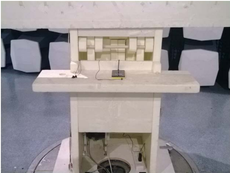
Picture 2. FCC Part 15B Radiated emissions
