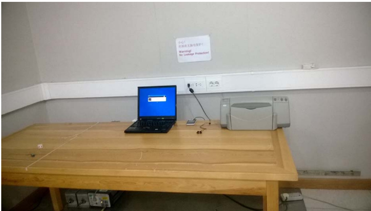
Picture 5. FCC Part 15B AC powerline conducted emissions, computer peripherals, measure from phone charger
