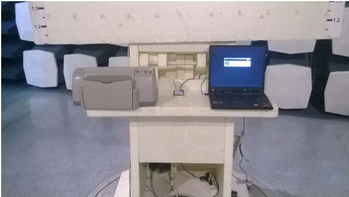
Picture 3. FCC Part 15B Radiated emissions, computer peripherals
