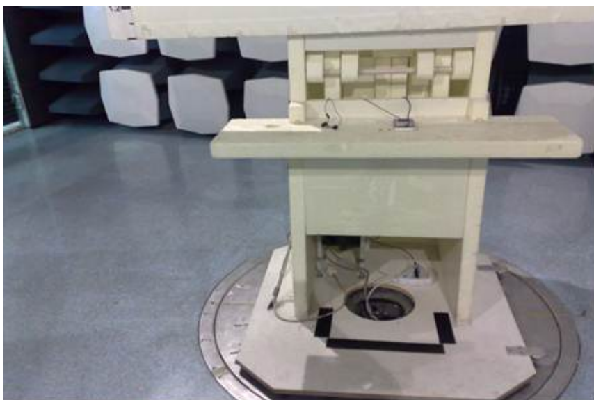
Picture 2. FCC Part 15B Radiated emissions
