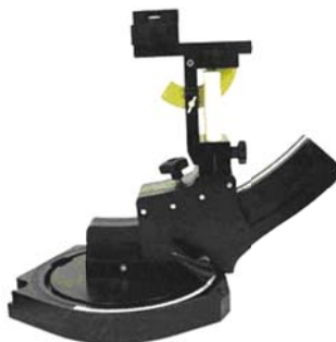
Device holder supplied by SPEAG
