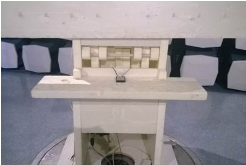
Picture 2. FCC Part 15B Radiated emissions
