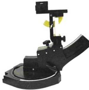
Device holder supplied by SPEAG
