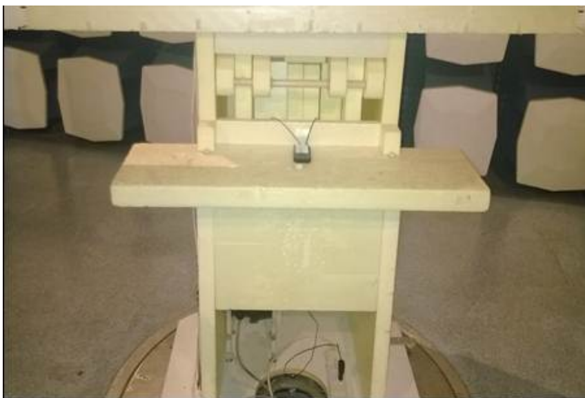
Picture 2. FCC Part 15B Radiated emissions
