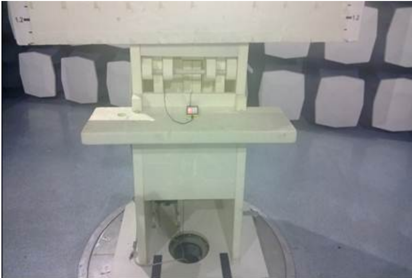
Picture 1. FCC Part 15C Radiated emissions
