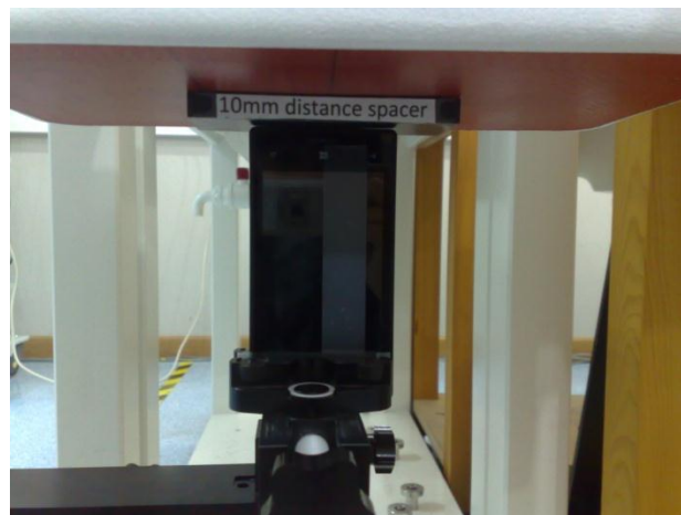
Photo of the device positioned for WR mode measurement – bottom edge facing phantom. The spacer was removed before the start of the measurements.
