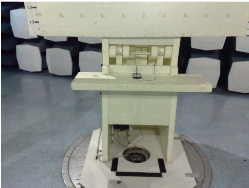
Picture 2. FCC Part 15B Radiated emissions
