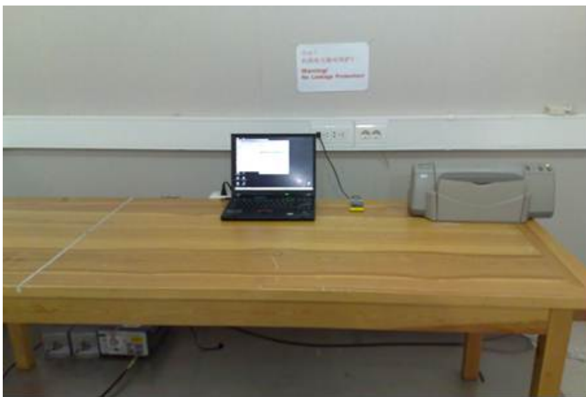
Picture 4. FCC Part 15B AC powerline conducted emissions, computer peripherals, measure from PC charger
