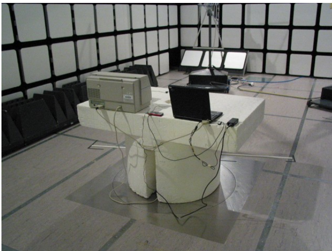
Picture 2. FCC Part 15B Radiated emissions
