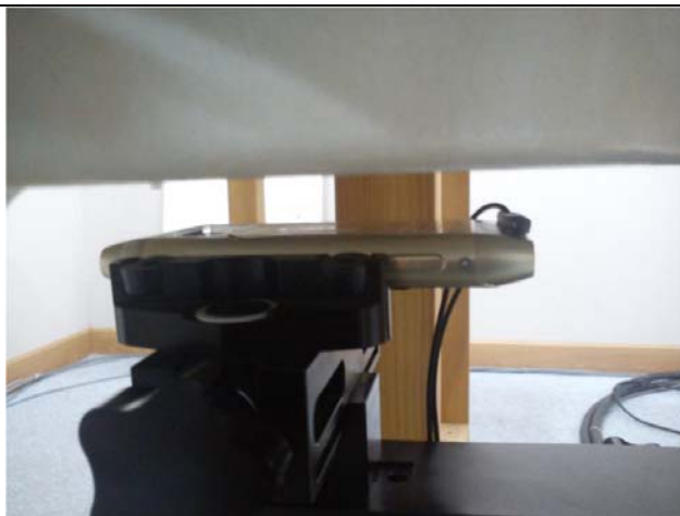
Photo of the device positioned for Body SAR measurement. Stylus Position 1
