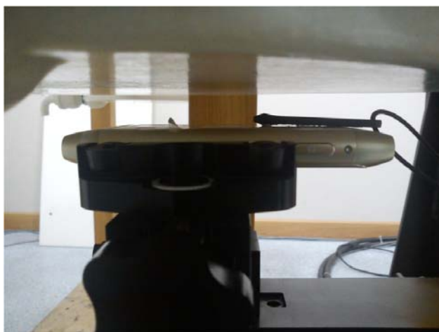
Photo of the device positioned for Body SAR measurement. Stylus Position 2
