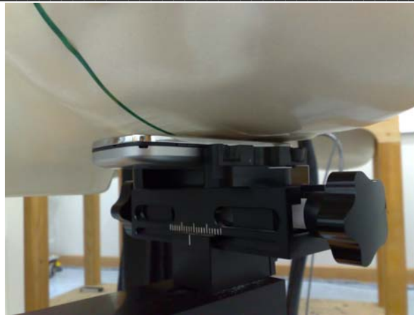
Photo of the device in “cheek” position
