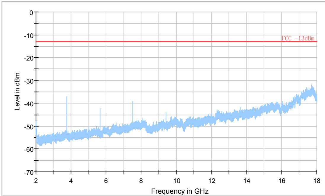
**A.2.4.6 RADIATED SPURIOUS EMISSIONS-Channel 810: 2GHz – 18GHz**
