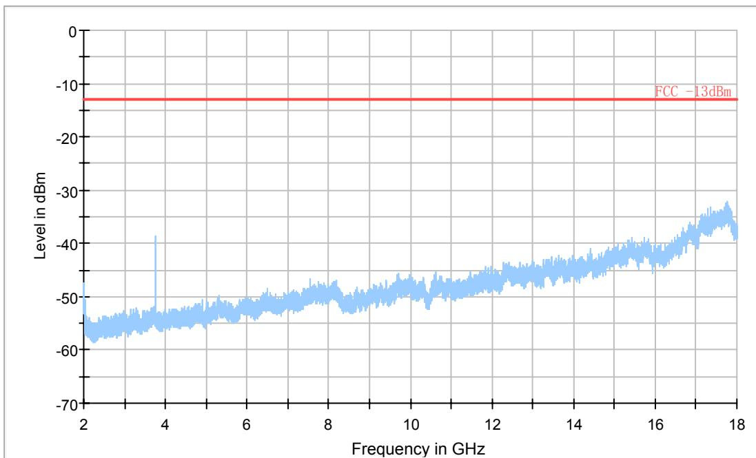
**A.2.4.16 RADIATED SPURIOUS EMISSIONS-Channel 810: 2GHz – 18GHz**
