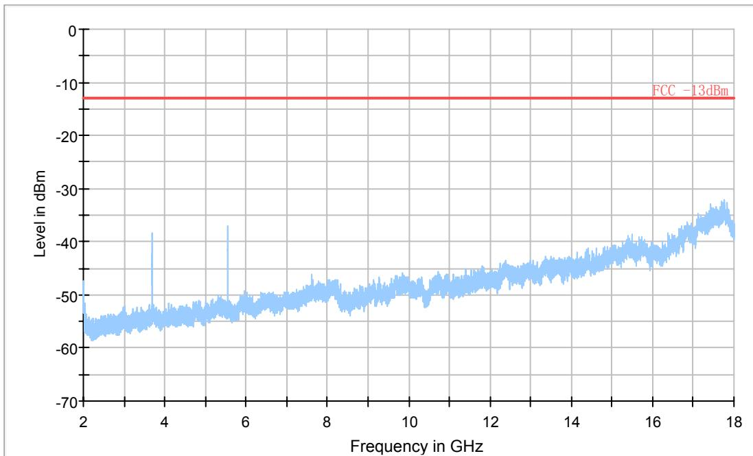
**A.2.4.15 RADIATED SPURIOUS EMISSIONS-Channel 661: 2GHz – 18GHz****Radiated spurious emission limit :-13dBm.**
