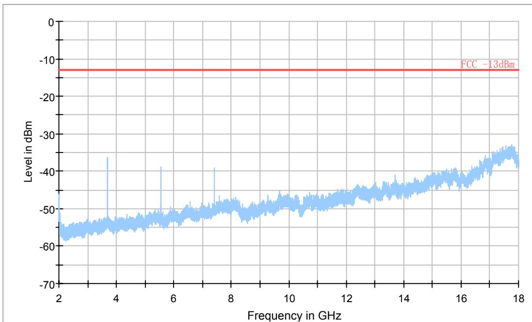
**A.2.4.5 RADIATED SPURIOUS EMISSIONS-Channel 661: 2GHz – 18GHz**
