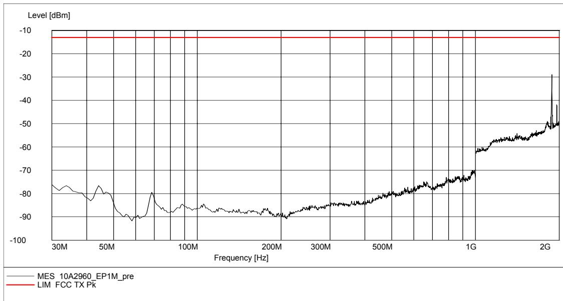
**A.2.4.13 RADIATED SPURIOUS EMISSIONS-Channel 810: 30MHz – 2GHz****Radiated spurious emission limit :-13dBm.****NOTE: peak above the limit line is the Carrier frequency @ ch-810**
