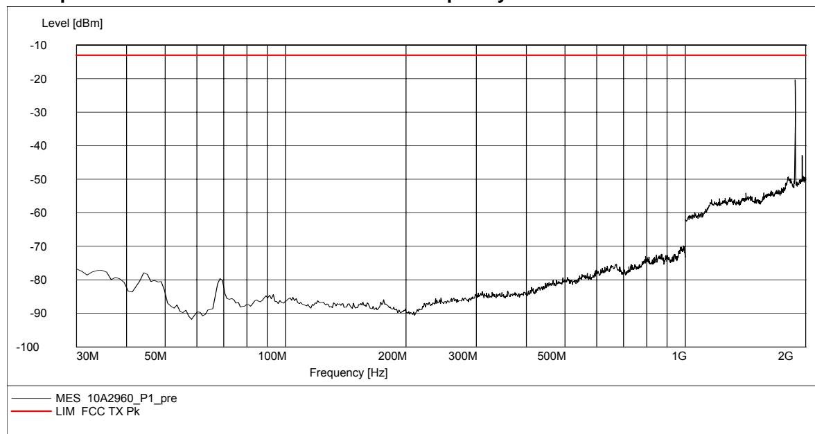
**A.2.4.3 RADIATED SPURIOUS EMISSIONS-Channel 810: 30MHz – 2GHz****Radiated spurious emission limit :-13dBm.****NOTE: peak above the limit line is the Carrier frequency @ ch-810**
