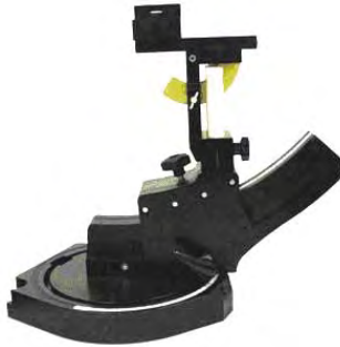
Device holder supplied by SPEAG
