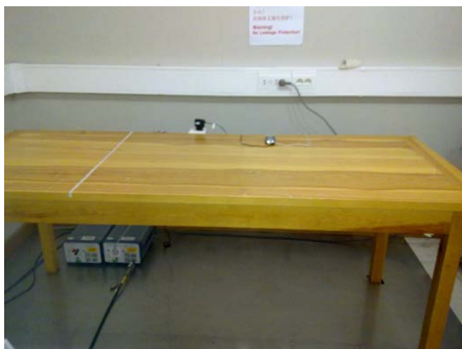
Picture 3 AC powerline conducted emission measurement 15C
