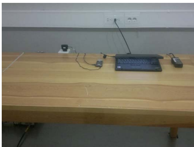
Picture 4 AC powerline conducted emission measurement 15B
