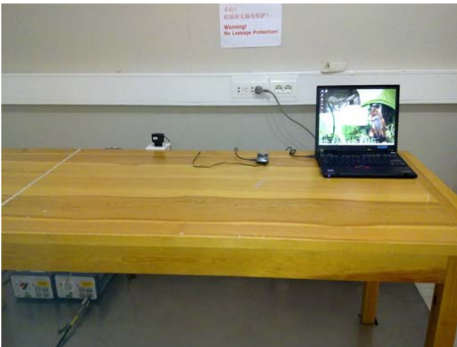
Picture 4 AC powerline conducted emission measurement 15B
