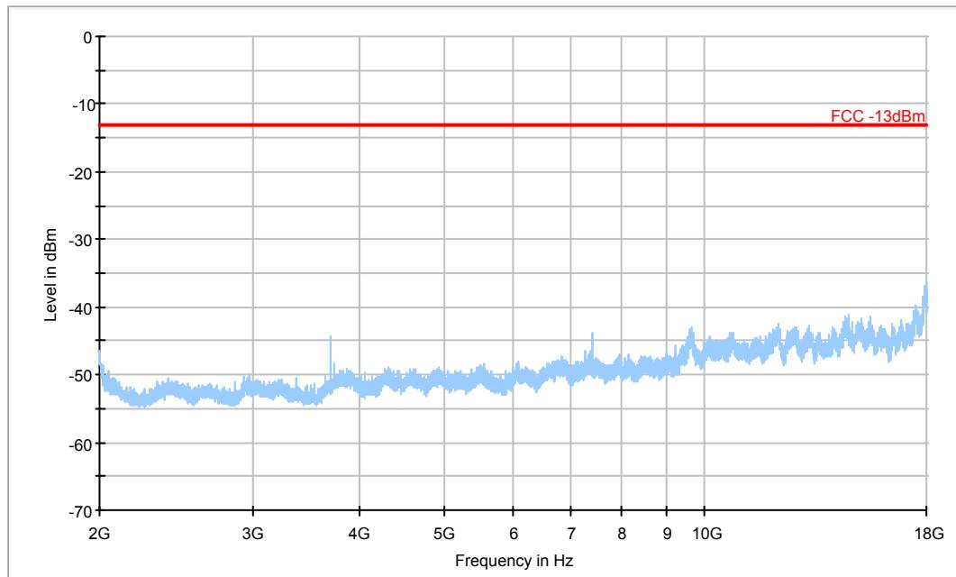
**A.2.3.5 RADIATED SPURIOUS EMISSIONS-Channel 661: 2GHz – 18GHz**
