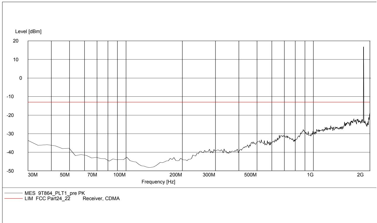
**A.2.3.2 RADIATED SPURIOUS EMISSIONS-Channel 661: 30MHz – 2GHz****Radiated spurious emission limit :-13dBm.****NOTE: peak above the limit line is the Carrier frequency @ ch-661**
