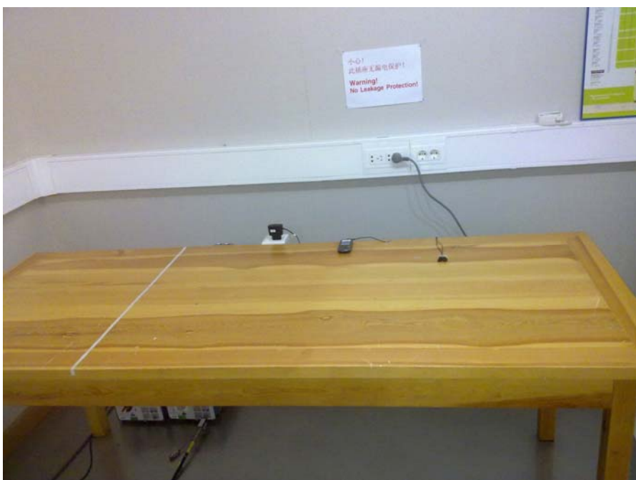
Picture 2 AC powerline conducted emission measurement 15C
