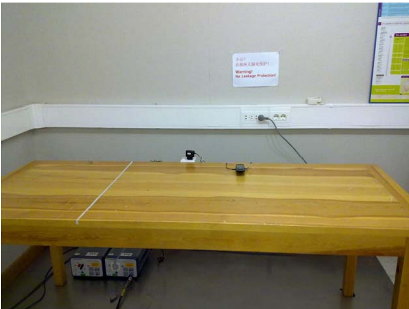
Picture 2 AC powerline conducted emission measurement 15C
