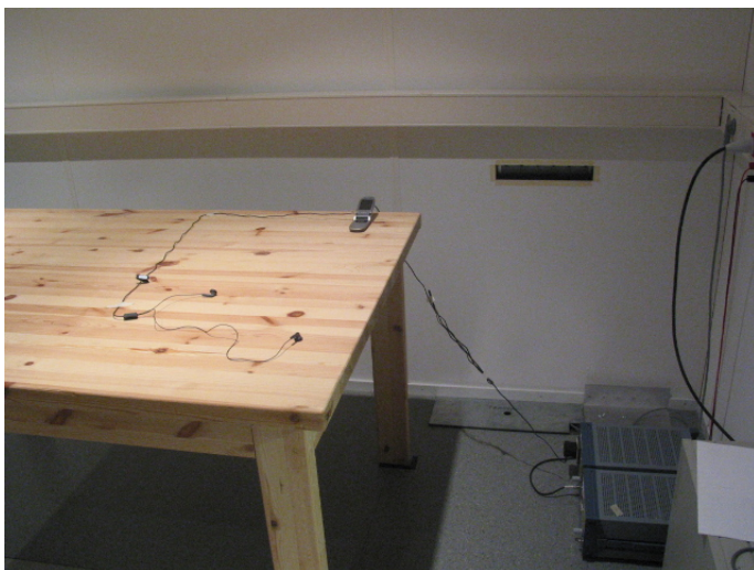
Picture 3 AC powerline conducted emission measurement GSM RX / Bluetooth TX
