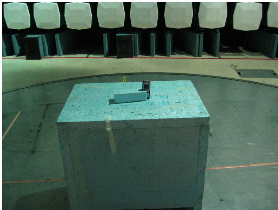
Photograph 1. Spurious radiated emissions test setup
