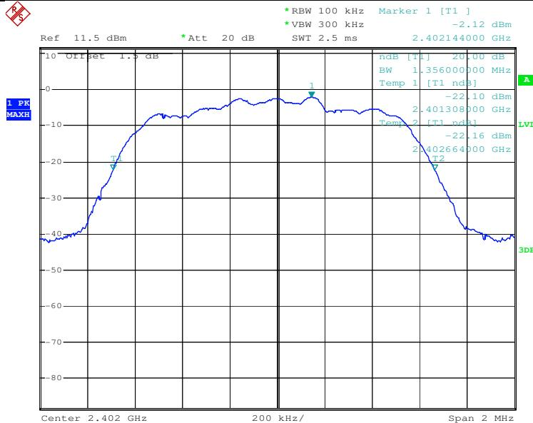
Test mode: 8DPSK Test channel: Highest
