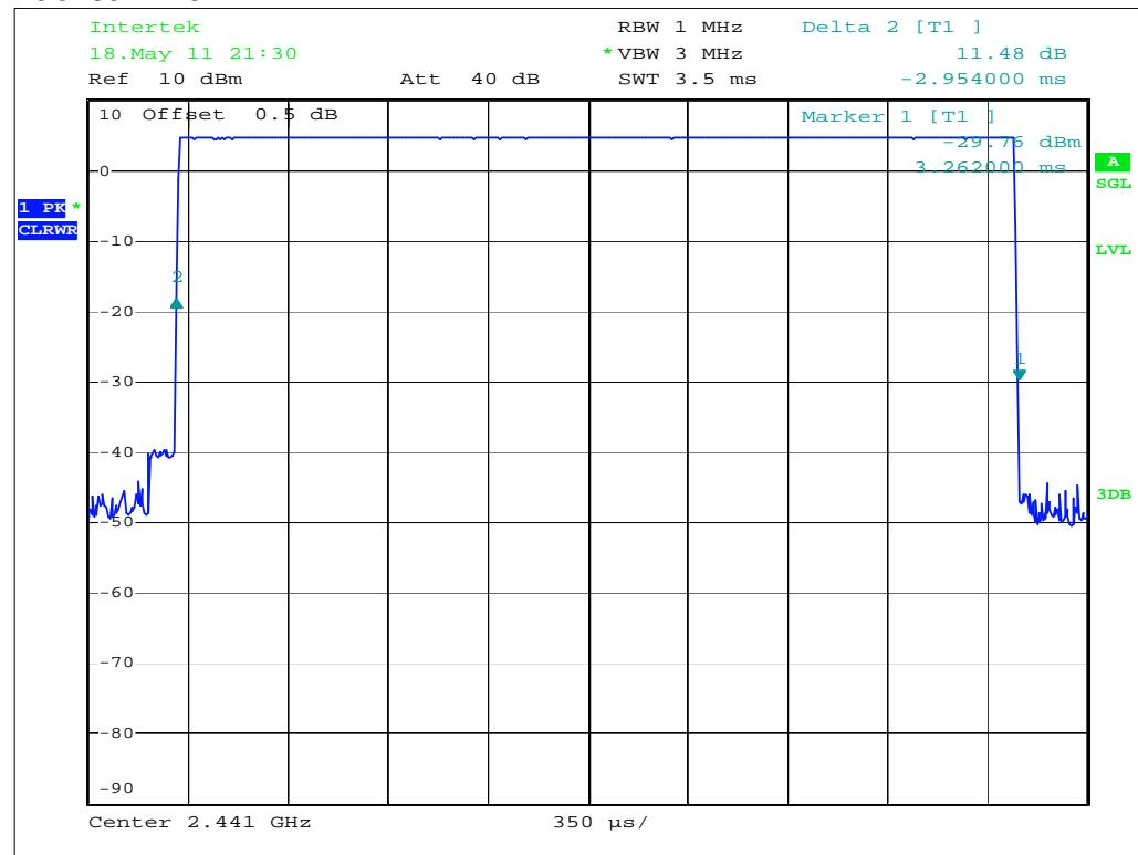
Modulation Type:  $\pi/4$  –DQPSK
