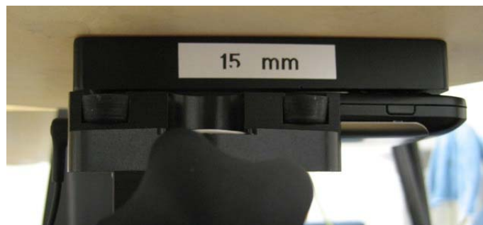
Photo of the device positioned for Body SAR measurement. The spacer was removed for the tests.
