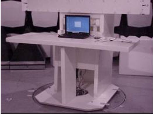
Picture 1. FCC Part 15C Radiated emissions
