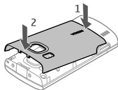
Always switch the device off and disconnect the charger before removing the battery.
