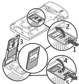
Ensure that the contact area on the card is facing down on the device, and
