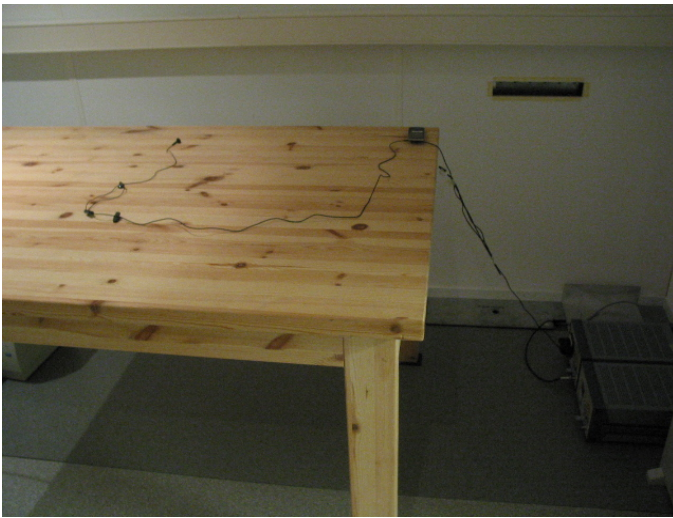
Picture 3 AC powerline conducted emission measurement
