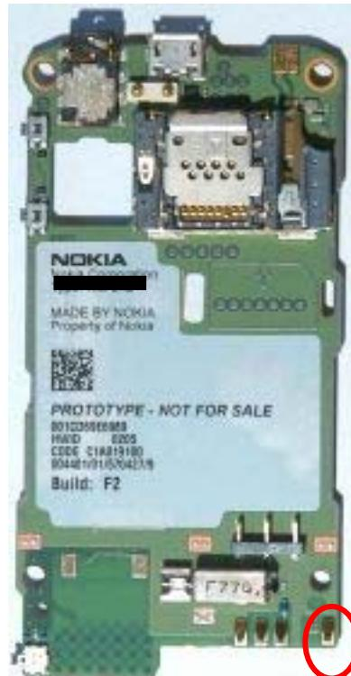
BT antenna contact to PWB
