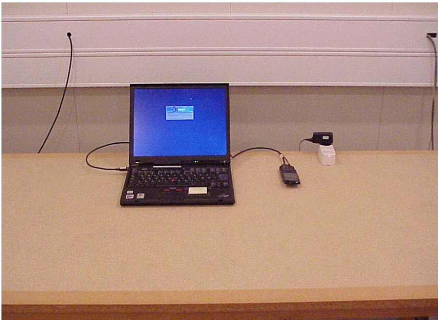
Picture 4 AC powerline conducted emission measurement GSM1900 RX and BT TX + Computer peripherals
